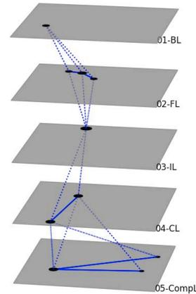
Fig. 8. SGAM-based NRGcoin exchange service mapped onto an MN. 01 – BL, 02 – FL, 03 – IL, 04 – CL and 05 – CompL correspond to business, function, information, communication and component layers respectively.
