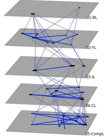
Fig. 7. SGAM-based NRG-X-Change architecture mapped onto an MN. 01 – BL, 02 – FL, 03 – IL, 04 – CL and 05 – CompL correspond to business, function, information, communication and component layers respectively.
