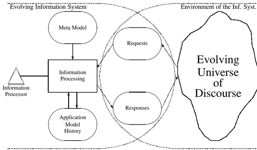
Figure 4: Evolving Information System Architecture
