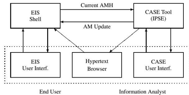
Figure 13: Hypertext Browser for an EIS-Shell and CASE-Tool
